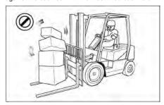
Do not lift or move loads that are not safe. Do not pick up an off center load. Such a load increases the possibility of a tipover to the side. Make sure loads are correctly stacked and positioned across both forks. Always use the proper size pallet. Position the forks as wide as possible under the load. Position loads evenly on the forks for proper balance. Do not lift a load with one fork.
