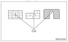
The point within an object, at which the whole weight of the object may be regarded as being concentrated, is called the center of gravity or CG. If the object is uniform, its geometric center will coincide with its CG. If it is not uniform, the CG could be at a point outside of the object. When the lift truck picks up a load, the truck and load have a new combined CG
