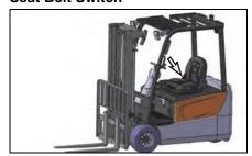
The seat belt switch is located next to the operator's seat.
