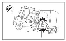
Do not operate on bridge plates unless they can support the weight of the truck and load. Make sure that they are correctly positioned. Put blocks on the vehicle you enter to keep it from moving.
