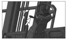
Move the directional control lever to the desired direction of travel.
