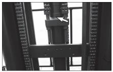
Inspect the chain anchors and individual links for wear, loose pins or cracked leaves.
