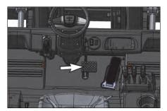
1. Apply the service brake to stop the lift truck.
