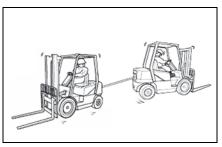
The counterweight draw bar should not be used for towing the forklift or for towing another forklift.
