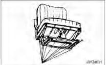
Check the operation of the seat adjusters. Make sure that the seat slides freely on its track. Lightly oil the seat slider tracks.
