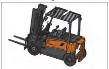
Lubricate fitting on steer axle.
