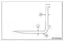
Check the fork blade (J) and shank (H) for wear with special attention to the heel (G). The fork should be withdrawn from service if the thickness is reduced to 90 percent or less of the original thickness.
