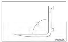
2. Check the angle between the upper face of the blade and the front face of the shank. The fork should be withdrawn from service if angle (C) exceeds 93 degrees or deviates by more than 3 degrees from an original angle other than 90 degrees, as may be found in some special application forks.
