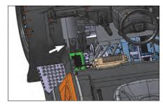
Check the pivot eye pins for loose retainer bolts and wear.
