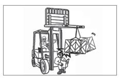
Carrying a load suspended on a chain or a cable may unbalance a truck.
