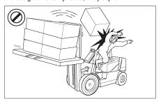
Do not operate your truck without the load backrest extension and overhead guard. Keep the load against the backrest with the mast tilted backward.
