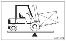
Counterbalanced lift truck design is based on the balance of two weights on opposite sides of a fulcrum (the front axle). The load on the forks must be balanced by the weight of the lift truck.
