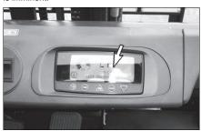
If the warning is ignored, lift interrupt will prevent the hydraulic pump motor from operating and an "EL" will be displayed on the LCD display.
