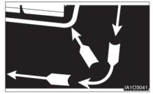
When turning in narrow aisles, keep as far from the stockpile as possible when making a turn into the aisle. Allow for counterweight swing.
