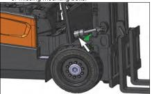
**8.** Inspect the hydraulic system for leaks, worn hoses or damaged lines.
