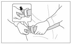
Push the button of the buckle to release the belt. The belt will automatically retract when released. Hold the plate of the belt and allow the belt to slowly retract.
