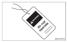
Attach a "Do Not Operate" or similar warning tag to start switch or controls before servicing or repairing the lift truck.
