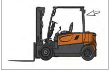
7. Inspect the overhead guard for damage, loose or missing mounting bolts.
