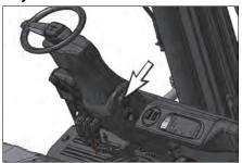
The key switch is located on the right side of the steering column.
