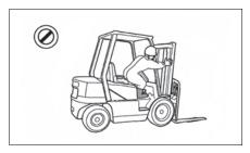
Do not operate a lift truck unless you are in the operator's seat. Keep hands and feet inside the operator's compartment. Do not put any part of the body outside of the operator's compartment. Never put any part of body into the mast structure or between the mast and the truck.
