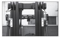
The channels on the roller-type mast require a break-in period. Apply a light film of lubricant on the channels where the rollers ride. This will prevent metal peel until the rollers set a pattern.
