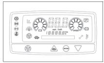
As you can see in Fig. on right side of display for type1 or type2 there are four keys: E-S-H, UP (TURTLE), DOWN and ENTER.
