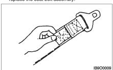
2. Belt Maintenance – Every 500 service hours. Check that the belt fastening works properly and that winding device is free from run lock when jerked. Check that the belt is suitably fastened to the seat. Check that the seat is correctly secured to the hood and the chassis. On visual inspection, fastenings must be intact, otherwise, contact the safety manager.
