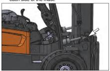
5. Check the mast pivot eye pins for loose retainer bolts and wear.
