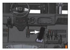
**Accelerator Pedal -** The accelerator pedal is located on the floor of the operator's compartment.
