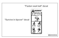
The "Survive in tipover" warning is located on the overhead guard. It shows the proper use of the operator restraint system.
