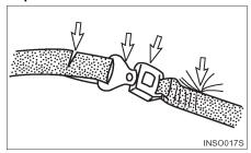
If the seat belt is torn, if pulling motion is interrupted during extension of the belt, or if the belt cannot be inserted into the buckle properly, replace the seat belt assembly.
