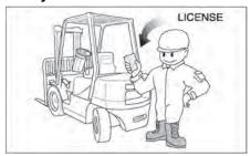
Only properly trained and authorized personnel should operate forklift trucks. Wear a hard hat and safety shoes when operating a lift truck. Do not wear loose clothing.
