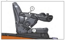
By using 2 knobs, adjust the position of the armrest to give the operator the best comfortable position of arm.
