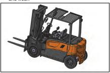
Lubricate the mast pivot eyes, one fitting on each side of the mast.
