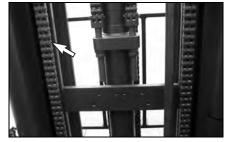
Inspect the part of the chain that is normally operated over the crosshead roller. When the chain bends over the roller, the movement of the parts against each other causes wear.
