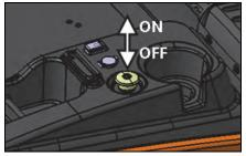
OFF - Push the emergency switch button to disconnect the electrical circuits. (It must be done after the key switch is turned off. If use often this button by the key switch, the electric system can make a problem. So, this button uses in emergency certainly).
