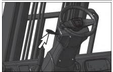
When directional control lever is equipped.
