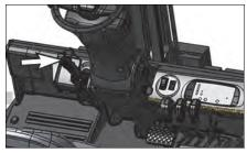
Engage the parking brake. (If equipped, Electric parking brake should be engaged. Please, refer next page.)
