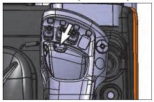
The auto tilt controller is at the rear side of the tilt knob. Press the auto tilt switch to turn on the switch lamp and push the tile knob forward. The mast will stop at 90 degrees angle.
