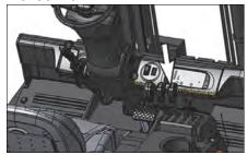
The sideshift attachment control is located at the operator's right side front. The sideshift attachment control lever is the lever at the right.
