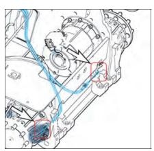
\*How to do EPB Forced Release temporarily – First, operate mast to secure a clear view of parking cable assembling in drive axle parking lever. Second, disassemble RH/LH parking cable from drive axle parking lever in the picture above and contact our service team.
