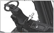
**4.** Turn the key switch to the ON position. Raise the attachments.
