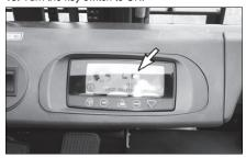
Check the LCD display for battery discharge status. A fully charged battery will be displayed on the LCD display.
