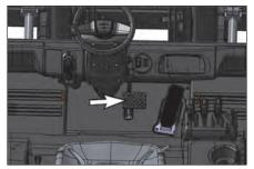
**Service Brake -** The service brake pedal is located on the floor of the operator's compartment.
