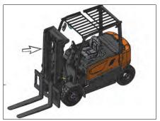
Fasten lift chains, of equal length, in lift openings in the front of the lift truck.
