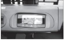
Check the indicator LCD display for the discharge state of the battery and the brake oil level
