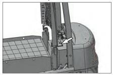
Loosen the bolts of the hydraulic tank top plate assembly.
