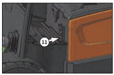
Inspect the battery compartment for loose connections, frayed cables and properly secured battery restraint.
