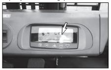
A fully charged battery will cause a "9 segments" to be displayed on the LCD display. As the battery is discharged, the LCD display will count down, 9, 8, 7, and etc., until "EL" is displayed. When the battery reaches 80% discharge level, the Micro-Controller will cause the LCD display to continuously index through the entire range (1 through 9 segments) to signal that the battery is discharged and lift interrupt is imminent.
