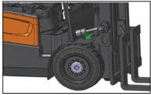
Inspect tires for wear, cuts, gouges and foreign objects. Look for bent rims and correct seating of locking ring.
