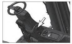
5. Turn key switch to OFF and remove the key.
