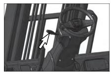
Move the directional control lever to the opposite direction of lift truck travel.
