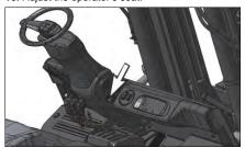
**11.** Adjust the steering wheel to a comfortable position.
