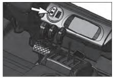
Parking Brake Engaged – Push the parking brake button (1), or when the operator leaves the seat, or there are no operational movements for 10 secs, which will engage the parking brake.
