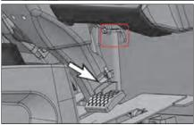
\*How to deal with Electric Parking Brake failure temporarily – First, Grab service pedal holding bracket locating under Instrument panel below. As picture, push the service brake pedal using the bracket and lock the pedal down using fixture marked as square in picture above and contact our service team.
