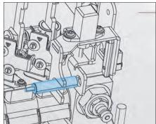
The lift neutral sensor is located in the main control valve at the bottom of the operating lever.
