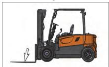
1. Lower the forks and tilt the mast forward.
