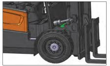
Park the lift truck level, with the parking brake engaged and directional control lever in NEUTRAL.
