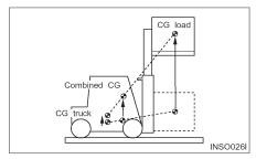
These same factors are also important for unloaded lift trucks. They tip over sideways easier than a loaded lift truck carrying its load in the lowered position.
