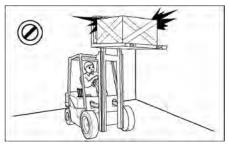
Look out for overhead obstructions when raising or stacking loads. Do not travel with a raised load. Do not travel with the mast raised. The lift truck can roll over and cause injury or death to you or other personnel.
