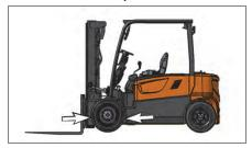
7. Block the wheels if parking on an incline.
