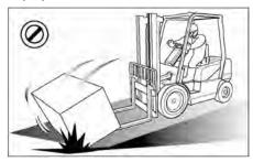
Go up ramps in forward direction and down ramps in reverse direction when moving loads.
