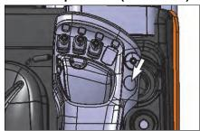
The auto clamp controller is at the rear side of the emergency switch. Pressing the auto clamp switch enables operation of the AUX2 knob. If not AUX2 operation signal is provided for 10 s after the trigger, the AUX2 will be locked. To reset the AUX2, press the auto clamp switch again. In addition, if no AUX2 operation signal is provided after key switch ON, the AUX2 will be locked up.
