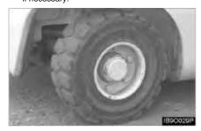
6. Install the steer wheel. Put two nuts opposite each other (180°). Tighten both. Install all remaining nuts. Tighten all nuts in a crisscross sequence opposite each other (180°) to a torque of 140 N·m (105 lb·ft).
