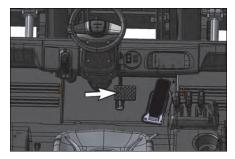
Push down on the service brake pedal and Prelease the parking brake.
