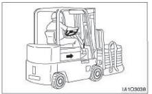
Carry the load as low as possible, while still maintaining ground clearance.
