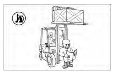
Do not permit anyone to stand or walk under the load or lifting mechanism. The load can fall and cause injury or death to anyone standing below.
