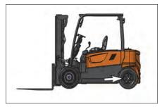
Inspect the tires, valve stems and wheels for cuts, gouges, foreign objects and loose or missing nuts. Refer to "Tires and Wheels" in "Every 10 Service Hours or Daily" section, if repairs or replacement is necessary.
