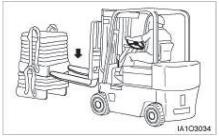
Move the lift truck forward until the load touches the carriage
