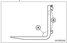
Forks should be inspected, at a minimum, every 12 months. If the truck is being used in a multi-shift or heavy duty operation, they should be checked every six months.
