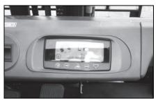
18. Make sure the battery is charged before operating the lift truck. A fully charged battery will cause "9 Segments" to be displayed on the BDI display.
