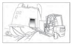
Be careful when operating a lift truck near the edge of a loading dock or ramp. Maintain a safe distance from the edge of docks, ramps and platforms. Always watch tail swing.
