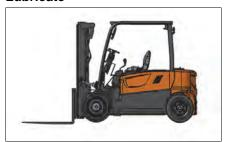
Operate the lift, tilt and attachment controls. Listen for unusual noises. These may indicate a need for repair.
