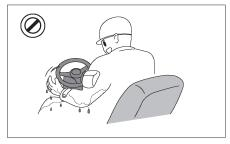
Never operate a lift truck with wet hands or shoes. Never hold any controls with grease on your hands. Your hands or feet will slide off of the controls and cause an accident.
