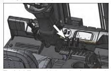
The forks' lift control is located at the operator's right side front. The lift control lever is the lever at the left.
