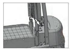
4. Remove the hydraulic filter and discard.
